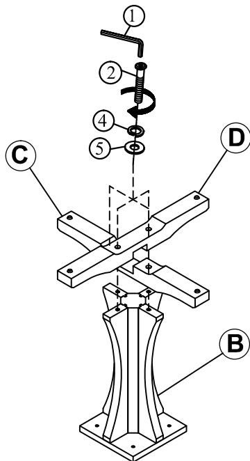
Step 2: Turn the Table Top (A) upside down on a soft surface such as a carpet and attach Pedestal (B) to Table Top (A) using Flat Washer (5). Spring Washer (4). Bolt (3) and tighten with Allen Key (1). Turn the table to upright position. Assembly is now complete. Thank you for your purchase.
